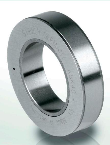
Type ASK is a roller type freewheel bearing supported by two rows of roller bearings. It is a self-contained dust protected unit, delivered grease lubricated.
